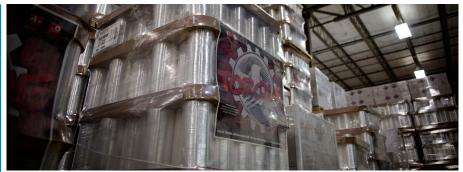
Holding force quantifies the amount of force the packaging applies to the load and vice versa. Stretch film provides a load-holding force far superior to that of other packaging materials.
